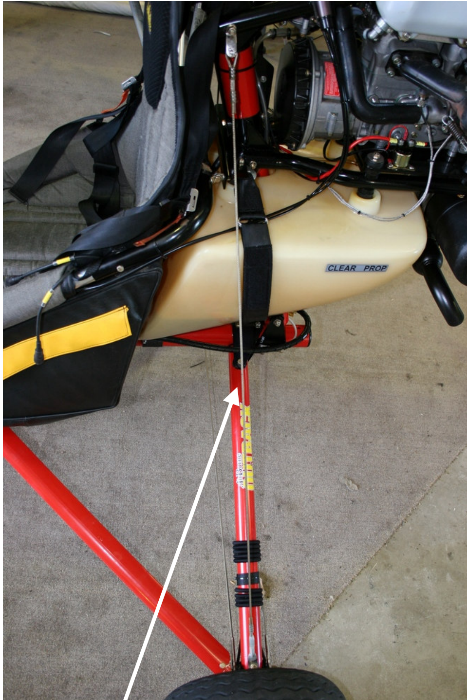
Figure 1 – Mast Support Wire X 1250, Part # 103070 as fitted to an Edge X Series Outback.
