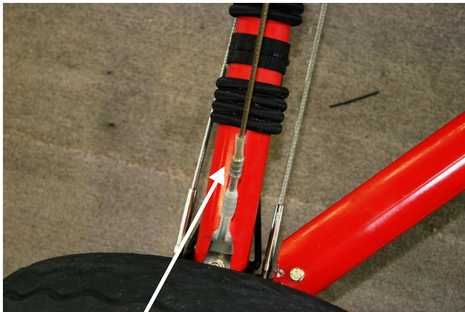
Figure 2 – Remove this heat shrink.
