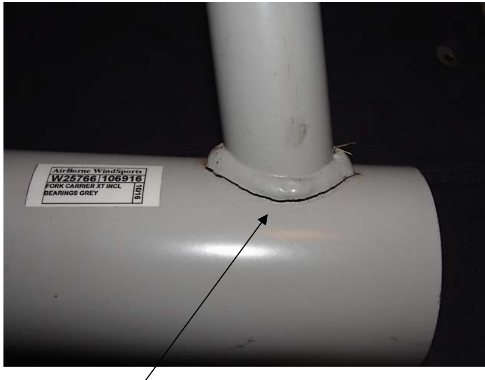
Figure 1 Cracking shown below weld
