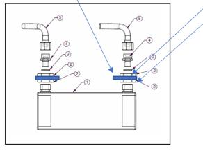
2017 versions and after require Spacer (Item 6 - Airborne Part #112990) and only one nut. Note orientation of spacer
