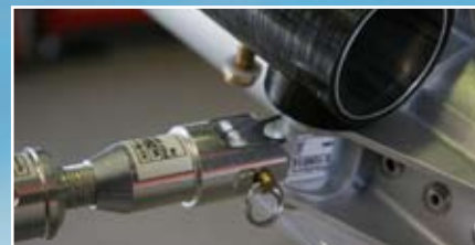
Crossbar leading edge junction with sprocket adjuster
