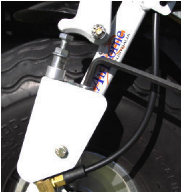
Figure 2 Brake master cylinder, remove reservoir plug
