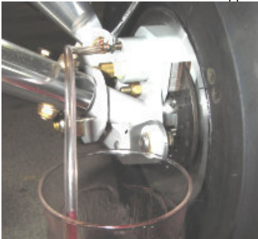
Figure 45 Bleed Drain Hose Connected
