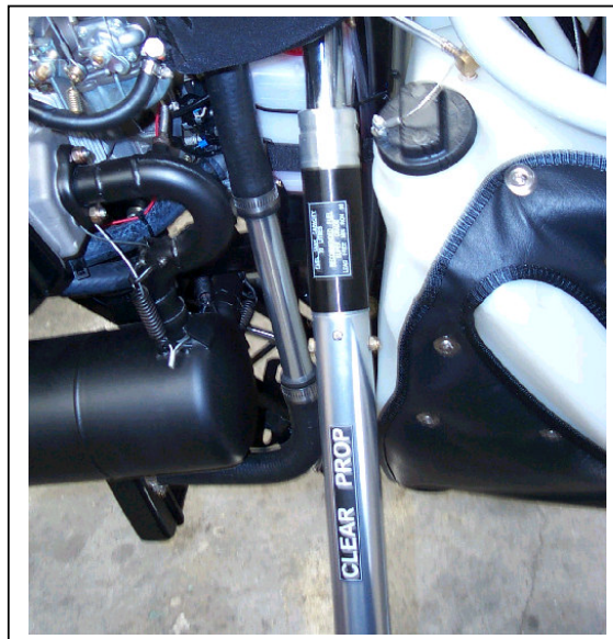
Figure 7 Section 2. Clear Prop and Fuel Spec Placards
