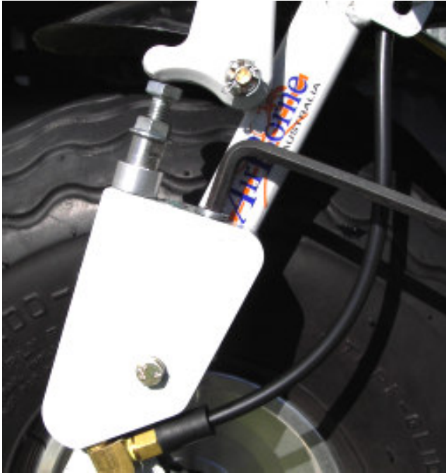
Figure 1 Brake master cylinder, remove reservoir plug
