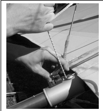
Figure 32 Section 4. De-tension Pull Back Cable
