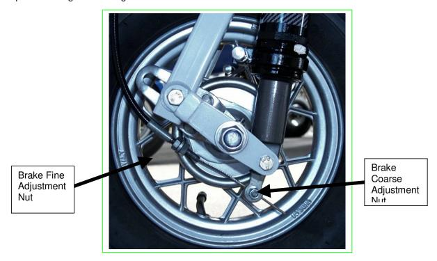
**Figure 29 Front Wheel Assembly**
