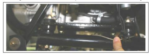
Figure 52 Engine Mount Rubbers (X 582 shown in photo)
