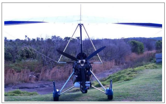
Figure 14 Parking Trike Tail to the Wind
