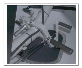
**Figure 33 Front Landing Gear Attachment**
