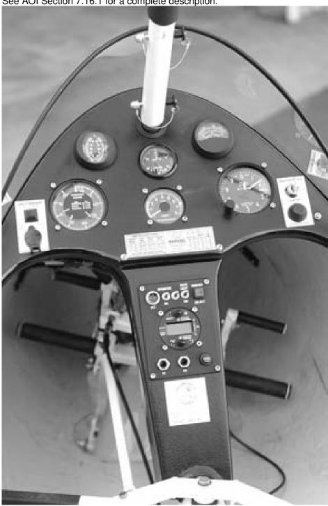
EGT, hour meter, water temperature
