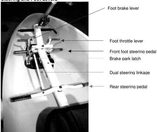
Figure 5 Steering and Foot Levers
