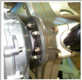
**Figure 48 Correctly Installed Propeller**
