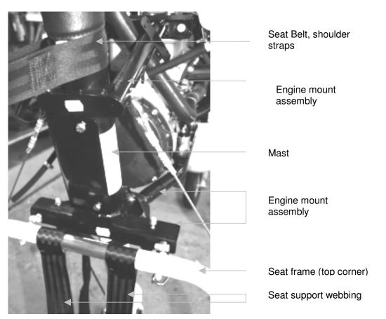
Figure 4 Mast Block Area (X Classic, partial assembly shown in photo)
