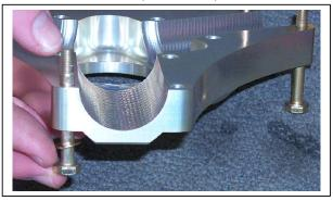
Figure 38 AN4 Bolts Into Forward Hub Block
