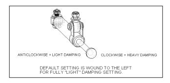
Figure 27 Steering Damper Setting
