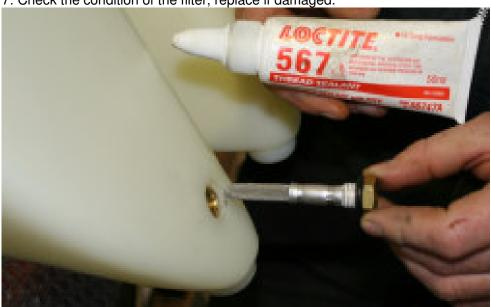
Figure 22 Finger Filter Installation
