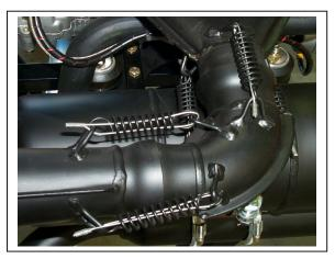
Figure 18 Muffler Safety Wire and Springs
