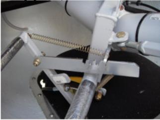
Figure 28 Brake Lock Lever.
