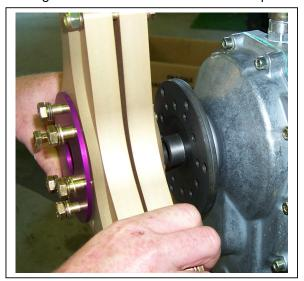
**Figure 41 Mounting the Propeller**
