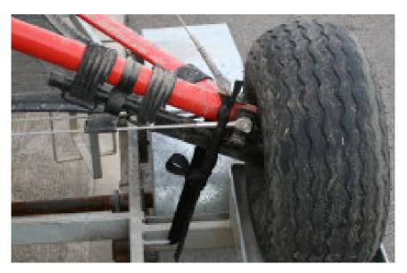
Figure 9 Rear Wheel Tie Down Location
