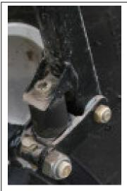
Figure 34 Front Fork to Wheel Attachment
