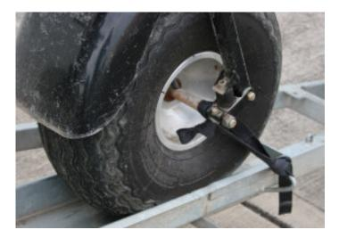
Figure 10 Front Wheel Tie Down
