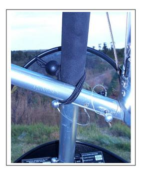
Figure 12 Parking of Trike (Upwind Wing Down)
