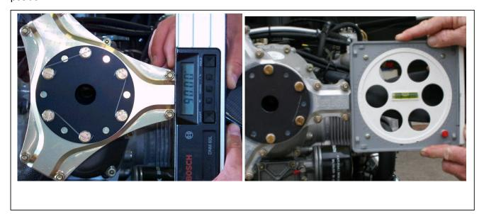
Figure 45 Propeller Horizontal Check
