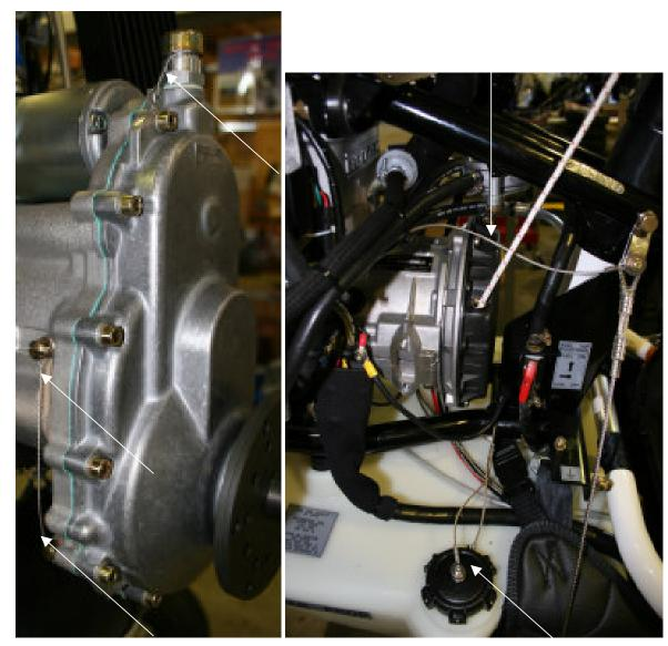
Figure 16 Tie Wire on Engine Gearbox
