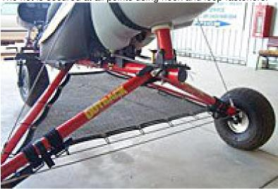
Figure 20 Propeller Net.
