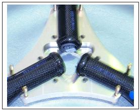
Figure 39 Place Blades into Hub Block
