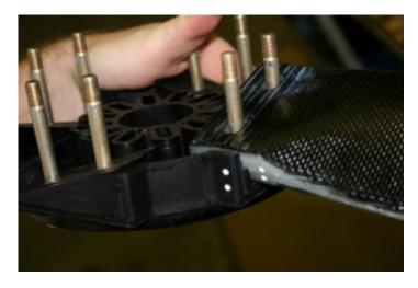
Figure 50 Install propeller blades
