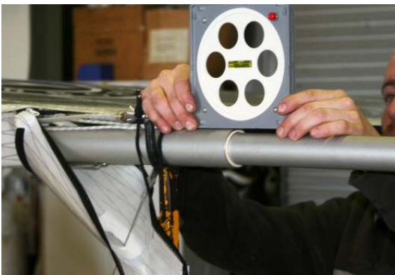
Figure 17 Setting Reference Keel Angle with protractor
