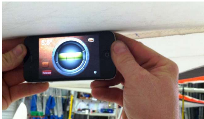
Figure 20 Measuring Washout Strut Angle with phone
