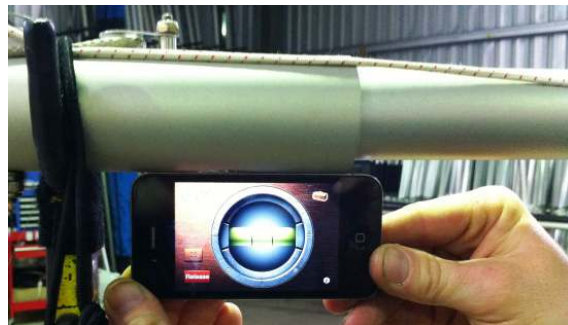
Figure 18 Setting Reference Keel Angle with phone
