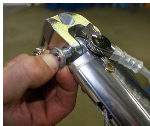
Figure 2 Section 5. Assemble control frame
