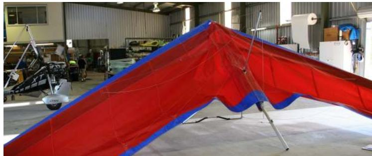
**Figure 5 Section 5. Raise king post and connect reflex bridle**
