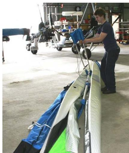
Figure 1 Section 5. Unzip wing bag
