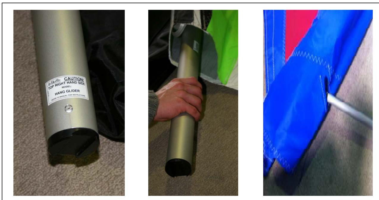
**Figure 11 Insertion of Rear Leading Edges**
