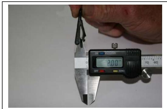
**Figure 15 Batten End Fitting Dimension Check**
