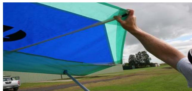
**Figure 9 Section 5. Install Washout Rod**
