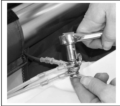
Figure 8 Removing top Front to Back Wire
