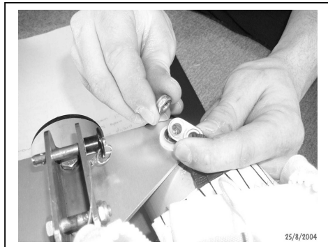
Figure 12 Removing nose webbing
