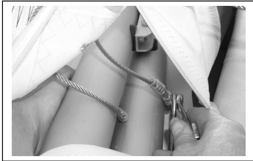
Figure 6 Unbolting Side Wires
