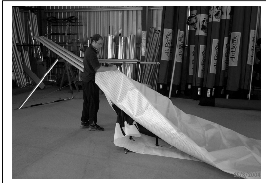
Figure 18 Sliding sail onto frame (Second Step)
