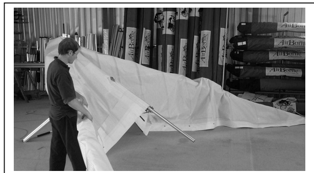
Figure 20 Position Keel pocket forward of rear wires
