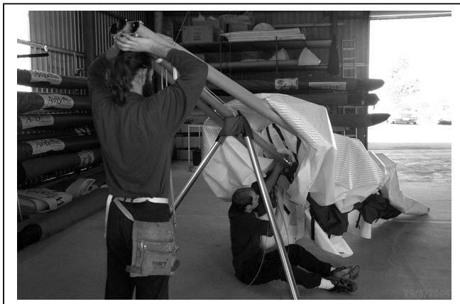
Figure 20 Position Keel pocket forward of rear wires
