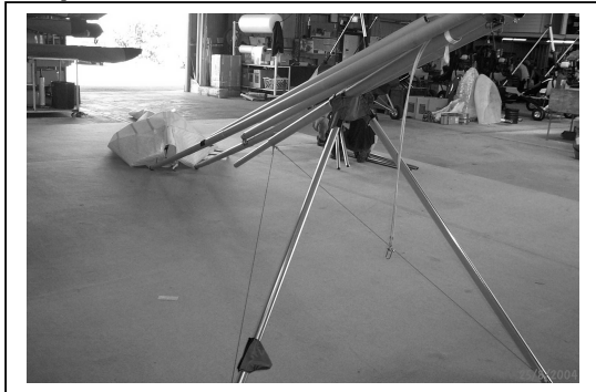
Figure 16 Frame preparation for Sail Reinstallation
