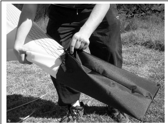
Figure 25 Section 4. Fit Tip Bags
