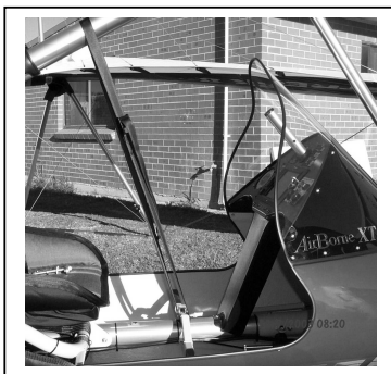
Figure 13 Section 4. Attach Mast Retaining Strap
