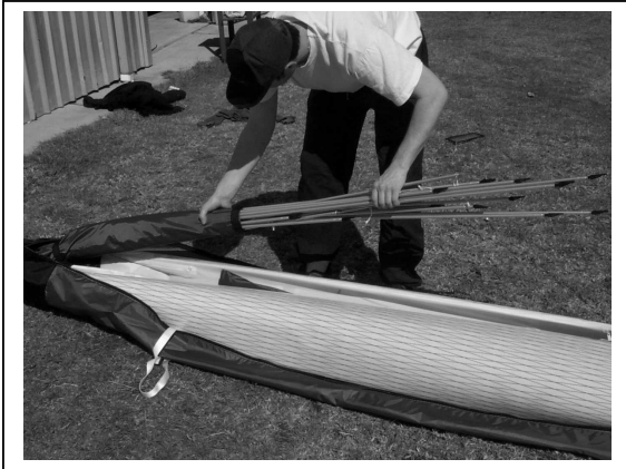
Figure 37 Section 4. Position Battens
