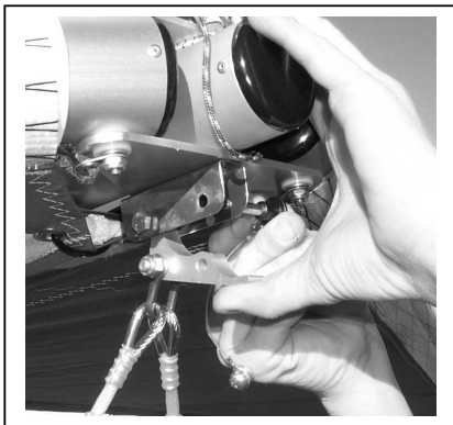
Figure 29 Section 4. Disconnect Nose Catch and Remove Nose Cone
