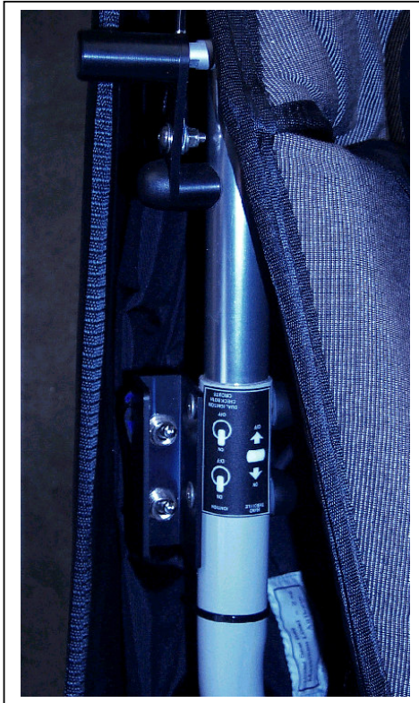
Figure 3 Section 2. Hand Throttle and Ignition Placard
