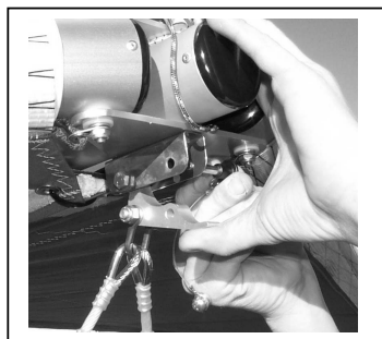
Figure 8 Section 4. Attach Nose Catch
