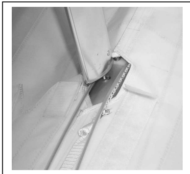
Figure 4 Section 4. Insert King Post
