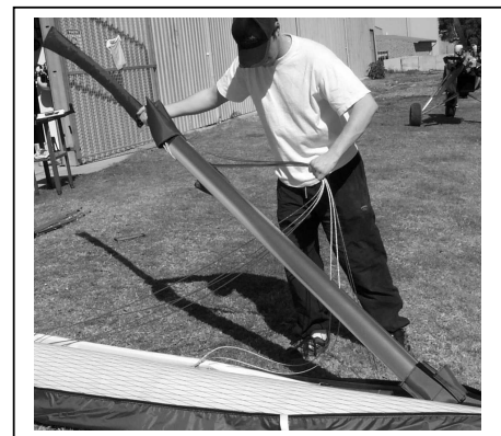
Figure 35 Section 4. Disconnect Base Bar
