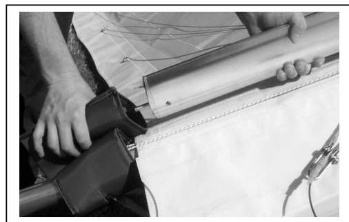
Figure 33 Section 4. Remove Kingpost
