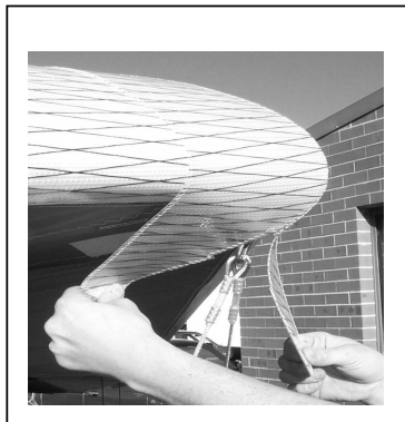
Figure 10 Section 4. Install Nose Fairing
