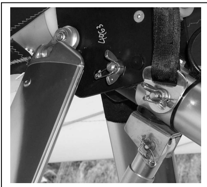
Figure 15 Section 4. Attach Wing to Wing U-Bracket
