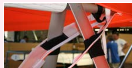
Keel pocket area unzipped for inspection
