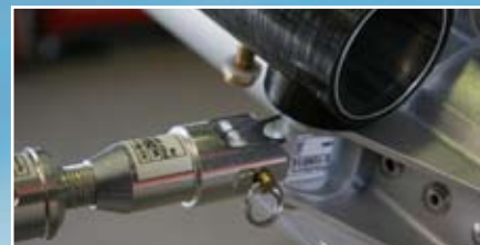
Crossbar leading edge junction with sprog adjuster
