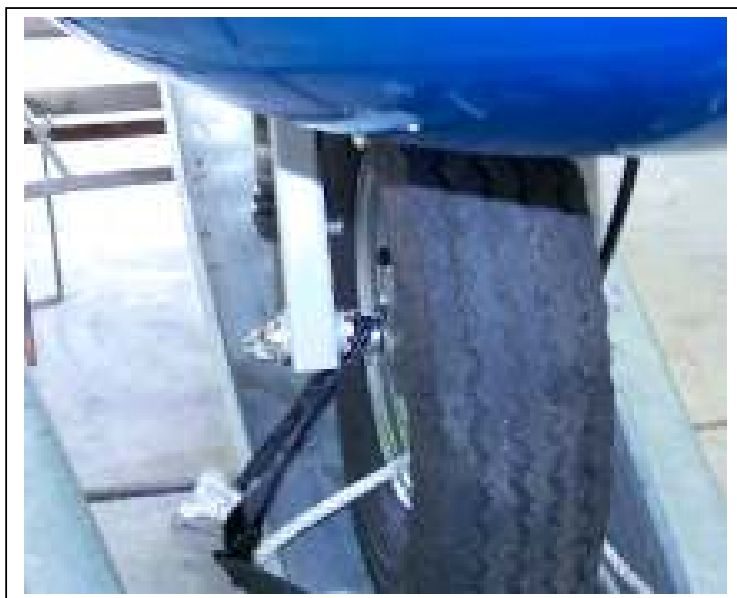
Figure 10 Front wheel with tie downs
