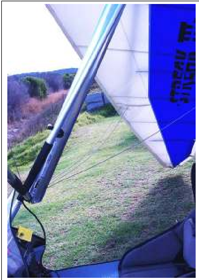
Figure 14 Securing of Base Bar With Bungee
