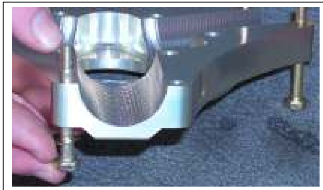
Figure 48 AN4 Bolts Into Forward Hub Block
