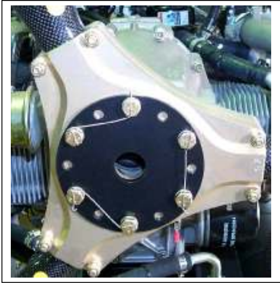
Figure 62 Correctly Installed Propeller
