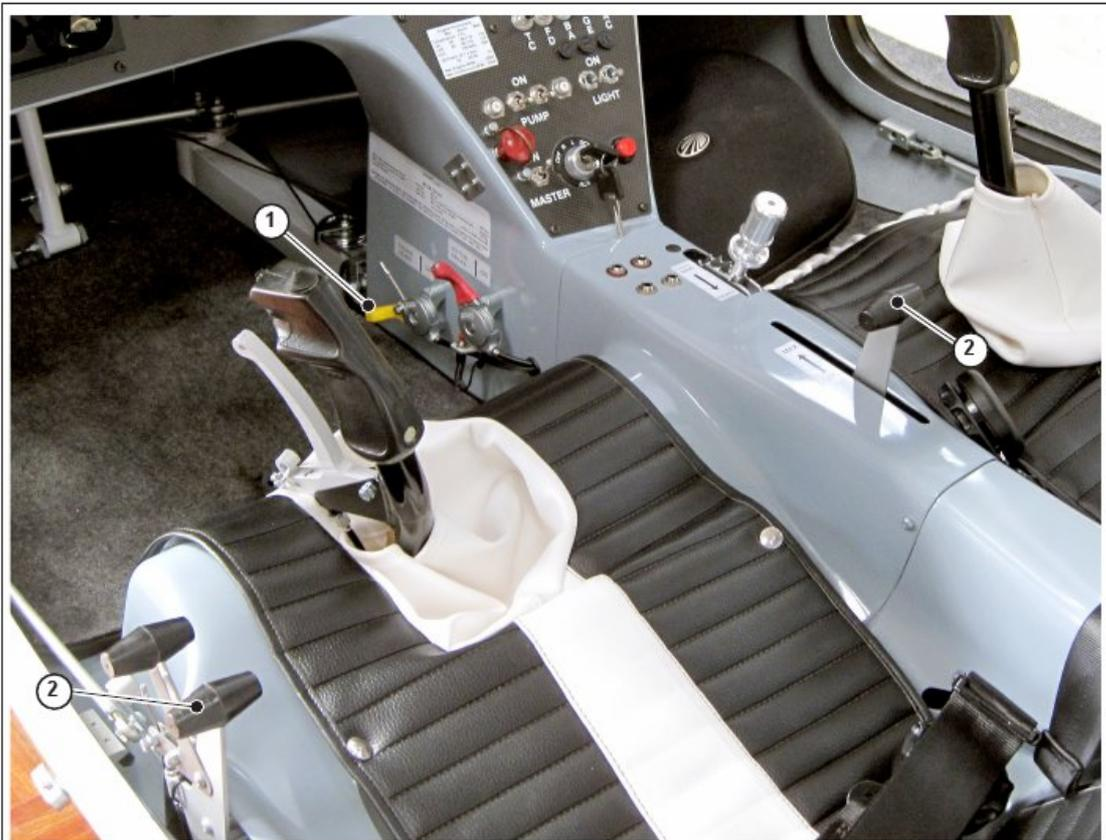
Fig.9 - Choke control lever
