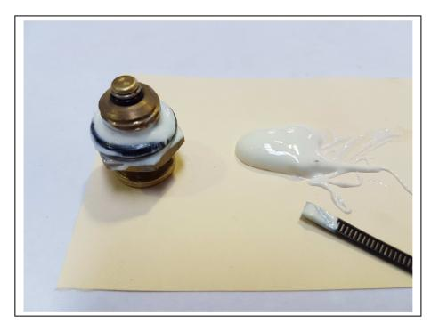
Refit Drain Cock slightly compressing "O" ring. JUST NOT LOOSE.
