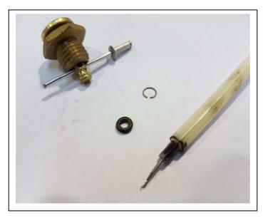
Compress spring in body and place sheer part of 1/8" rivet or similar in cross holes to hold spring compressed. SEE PHOTO.
