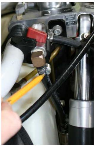
4/ ATTACH FUEL SENDER TO THE 60L HOSES. Attach the 60L hose coming from the kit to the INLET of the fuel sender, and the loose 60L hose to the OUTLET of the sender.
