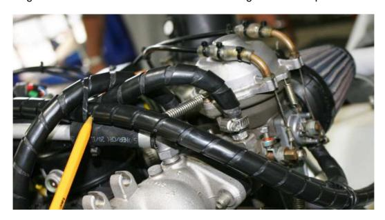
11/ RECONNECT THE FUEL FLOW SENDER TO THE TOP LINK MODULE. Route the sender wire under the equalizer and fuel hoses and reconnect to the engine sender module, black wire to GND, red wire to RD, blue wire to BL.
