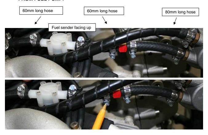
Using a medium cable tie secure the fuel sender to the fuel pump intlet line.
