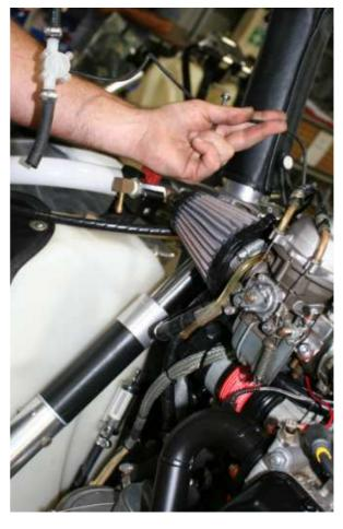
3/ INSTALL 215L HOSE. Using the existing hose clamps, install the 215L hose from the fuel tap elbow to the fuel filter. Note: Face the hose clamps outwards to the rear wheel for ease of access.
