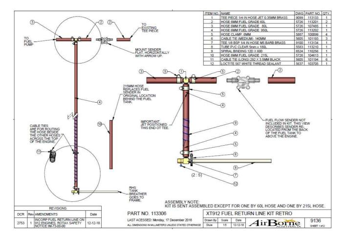
The drawing shows the kit as it should be received, the parts referred to in this Service Bulletin, and some fitting comments.
