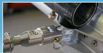
Crossbar leading edge junction with sprog adjuster
