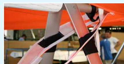
Keel pocket area unzipped for inspection
