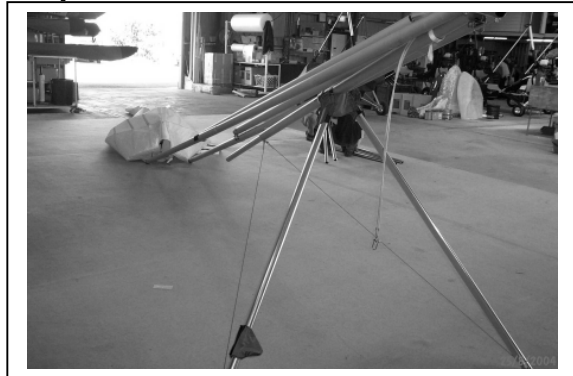
Figure 16 Frame preparation for Sail Reinstallation
