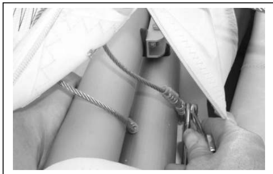
Figure 6 Unbolting Side Wires
