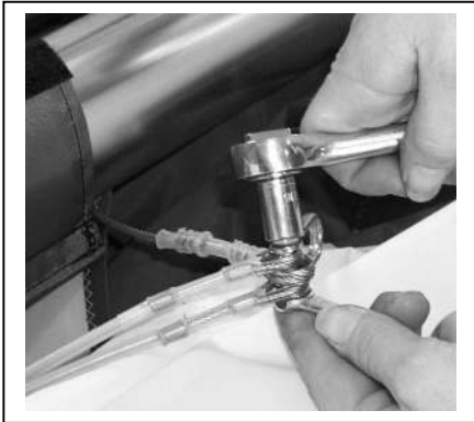
Figure 8 Removing top Front to Back Wire
