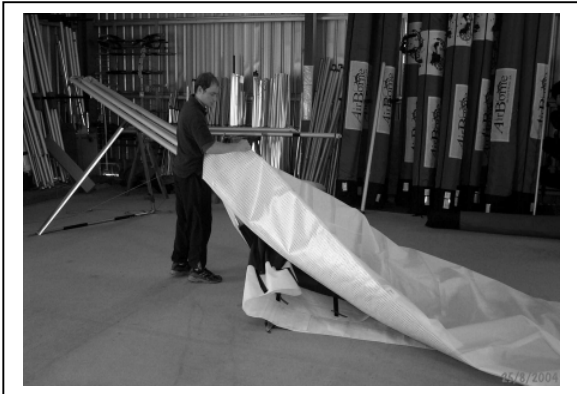
Figure 18 Sliding sail onto frame (Second Step)
