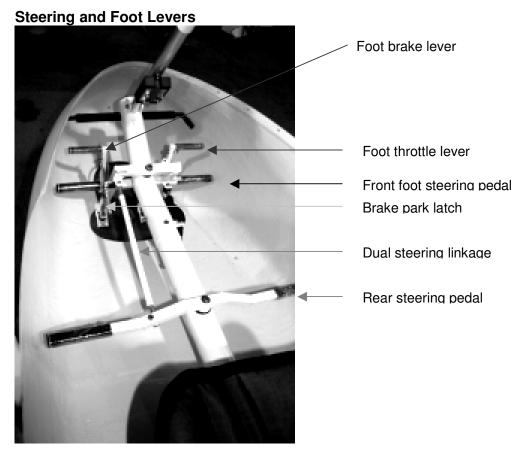
Figure 5 Steering and Foot Levers
