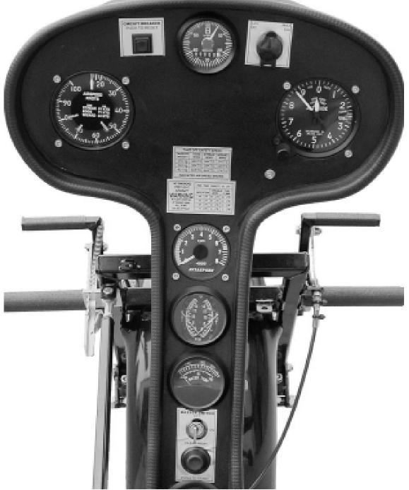
Top Row L to R:Circuit Breaker, Hour Meter, Power Outlet2<sup>nd</sup> top Row L to R:ASI, AltimeterVertical column top to bottom:Tachometer, EGT, Water Temperature, Instrument Power Switch, ElectricStart.
