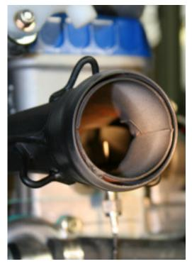
Figure 54 Installation of EGT Sender
