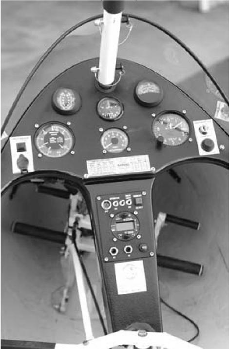
Top Row L to R: 2<sup>nd</sup> top Row L to R: EGT, hour meter, water temperature Circuit breaker, Power Outlet, ASI, Tachometer, Altimeter, Instrument Power Switch, Electric Start. Radio.
