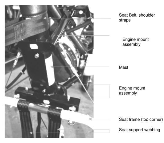
Figure 4 Mast Block Area (X Classic, partial assembly shown in photo)
