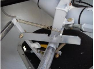
Figure 28 Brake Lock Lever.
