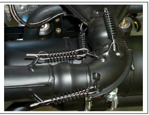
Figure 18 Muffler Safety Wire and Springs
