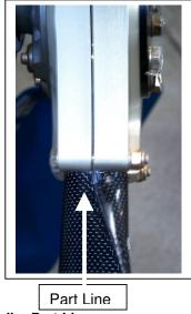
Figure 43 Propeller Part Lines
