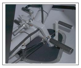
Figure 33 Front Landing Gear Attachment
