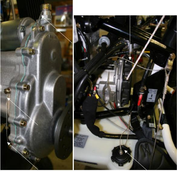
Figure 16 Tie Wire on Engine Gearbox
