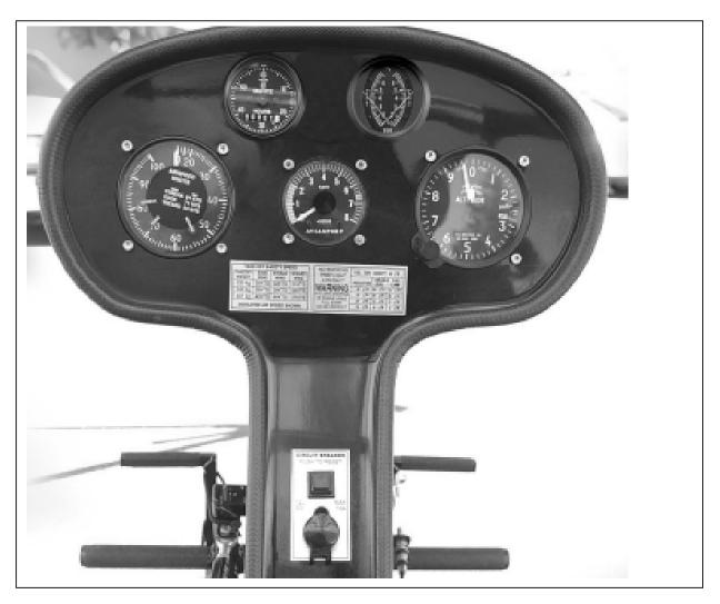
Top row L to R:hour meter, CHTBottom Row L to R:ASI, Tachometer, AltimeterBottom:Circuit breaker, power outlet
