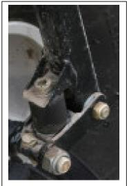
Figure 34 Front Fork to Wheel Attachment
