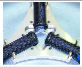
Figure 39 Place Blades into Hub Block
