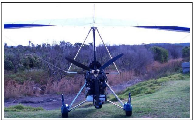
Figure 14 Parking Trike Tail to the Wind
