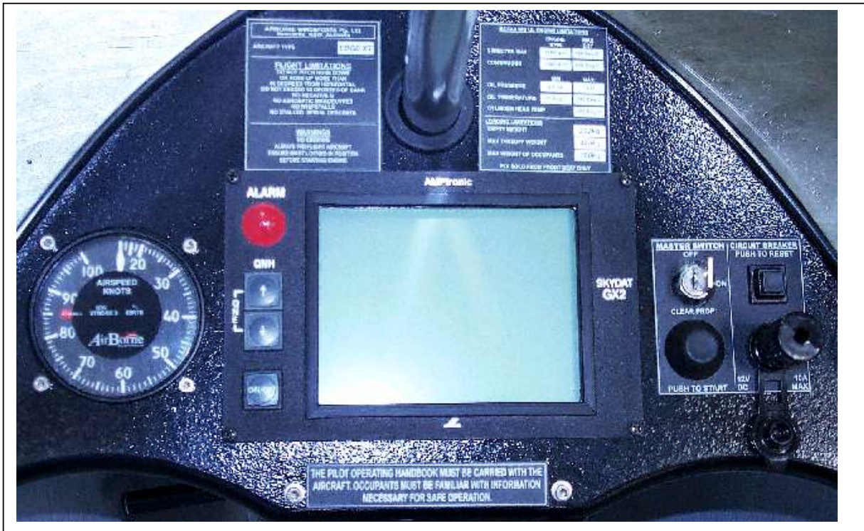
Figure 1 Section 2. Flight Limitations, Airspeed, Circuit Breaker, Power Socket and Aircraft Operating Instructions Placard Locations
