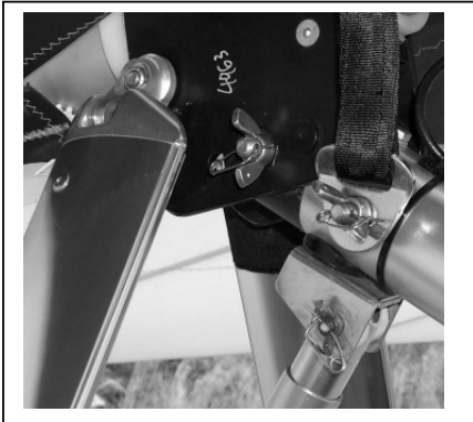
Figure 16 Section 4. Attach Wing to Wing U-Bracket
