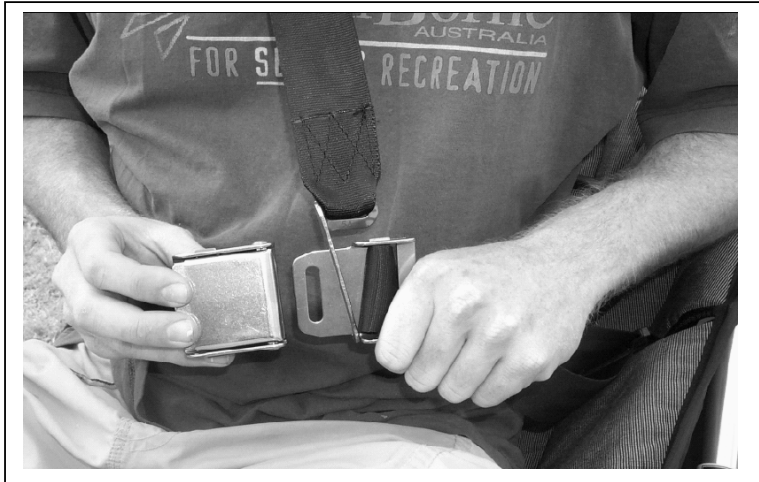
Figure 2 Section 7. Fastening Seat Belt with Shoulder Sash.
