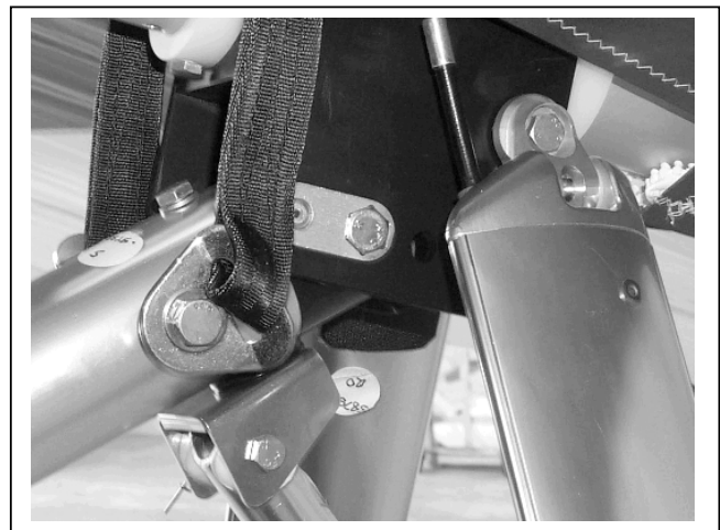
Figure 17 Section 4. Heart Bolt Retainer Position
