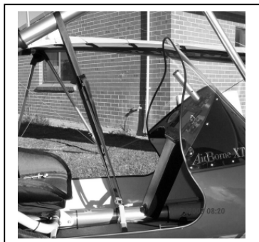
Figure 14 Section 4. Attach Mast Retaining Strap
