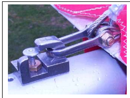
Figure 6 Section 4. Tensioning Cross Bar and Shackle Located in Block.
