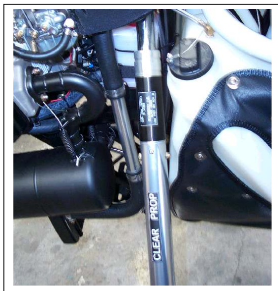
Figure 6 Section 2. Clear Prop and Fuel Spec Placards
