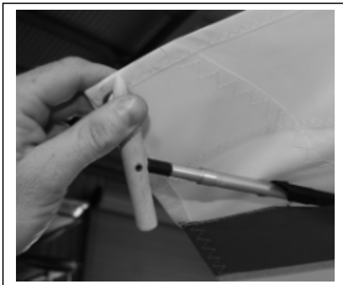
Figure 60 Section 4. Detension Tip Strut
