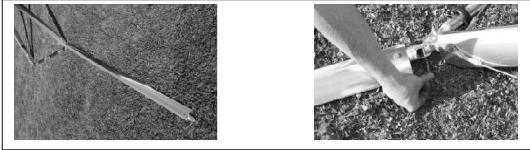
Figure 16 Section 4. Connect Control Frame To Wing Struts
