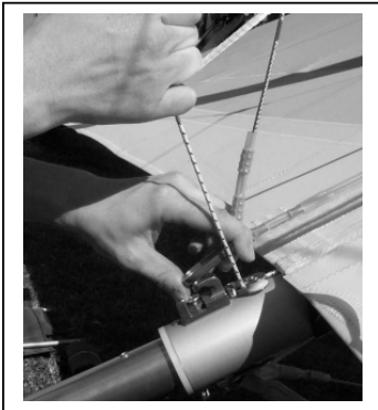
Figure 51 Section 4. De-tension Pull Back Cable
