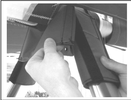
Figure 47 Section 4. Velcro U-Bracket Face Cover
