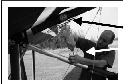
Figure 31 Section 4. Attach Trimmer to Mast
