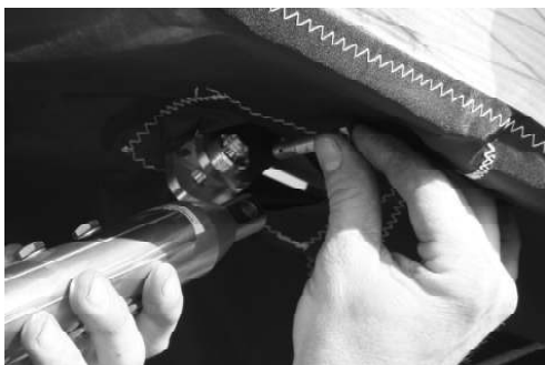
Figure 67 Section 4. Remove Strut to Leading Edge Connecting Bolt
