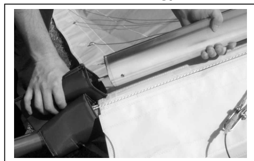
Figure 53 Section 4. Remove Kingpost
