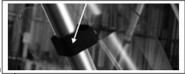
Figure 36 Section 4. Secure Windscreen XT 880mm
