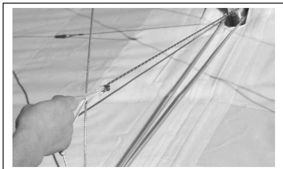
Figure 19 Section 4. Tensioning Cross Bar and Shackle Located in Block.
