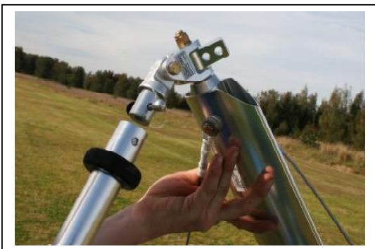
Figure 72 Section 4. Disconnect Base Bar
