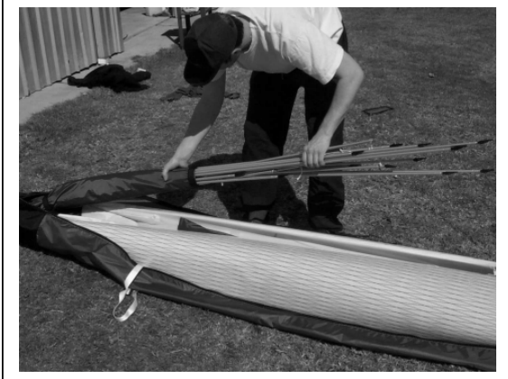
Figure 57 Section 4. Position Battens
