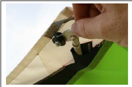
Figure 59 Section 4. Unload Over-Centre Tip Battens
