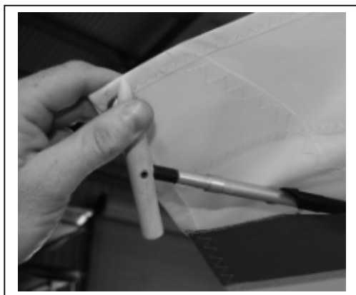
Figure 41 Section 4. Detension Tip Strut
