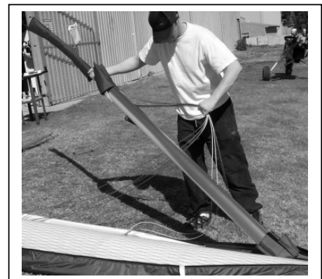
Figure 55 Section 4. Disconnect Base Bar
