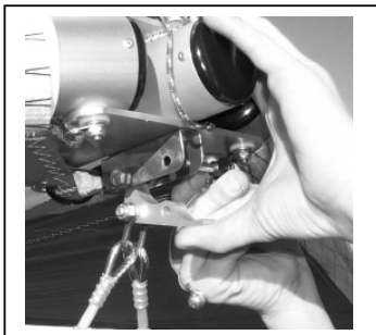
Figure 8 Section 4. Attach Nose Catch
