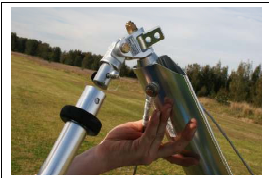
Figure 72 Section 4. Disconnect Base Bar
