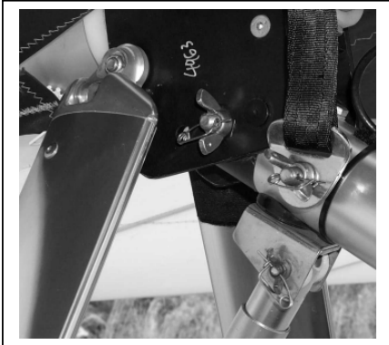
Figure 29 Section 4. Attach Wing to Wing U-Bracket
