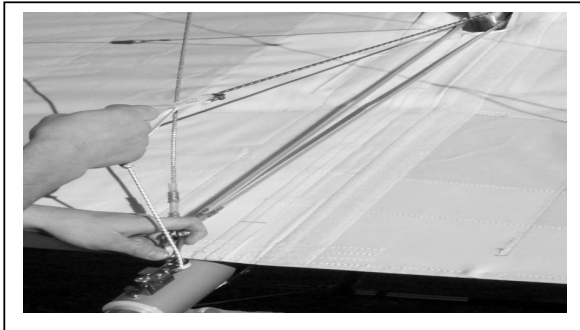
Figure 6 Section 4. Tensioning Cross Bar and Shackle Located in Block.
