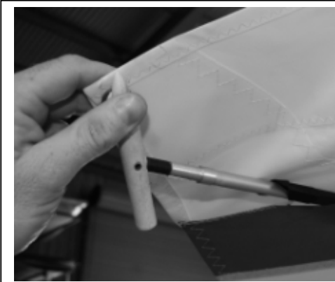
Figure 60 Section 4. Detension Tip Strut
