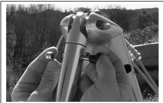
Figure 55 Section 4. Disconnect Base Bar
