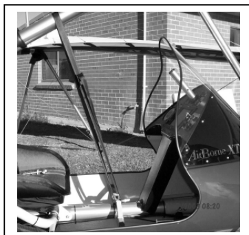
Figure 27 Section 4. Attach Mast Retaining Strap
