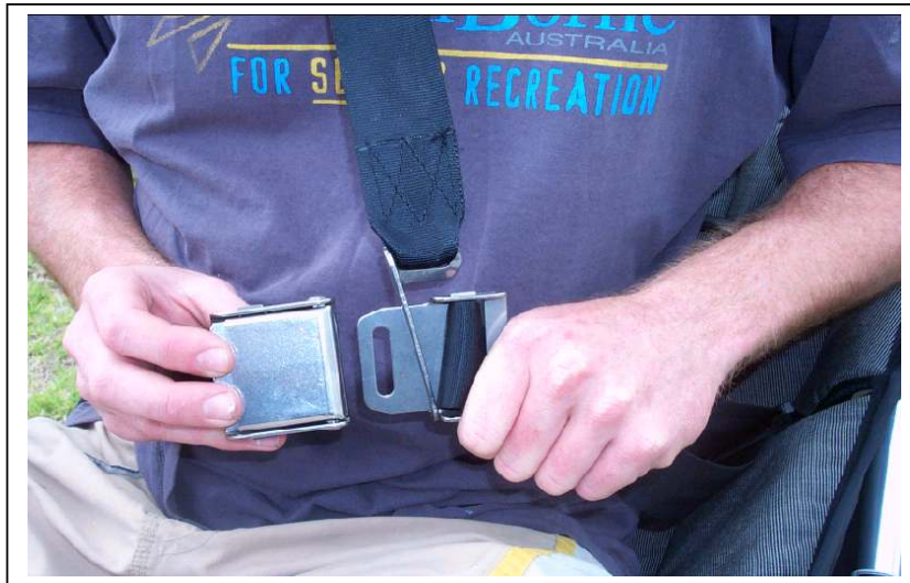
Figure 2 Section 7. Restraint harness, shoulder sash & buckle fitting.
