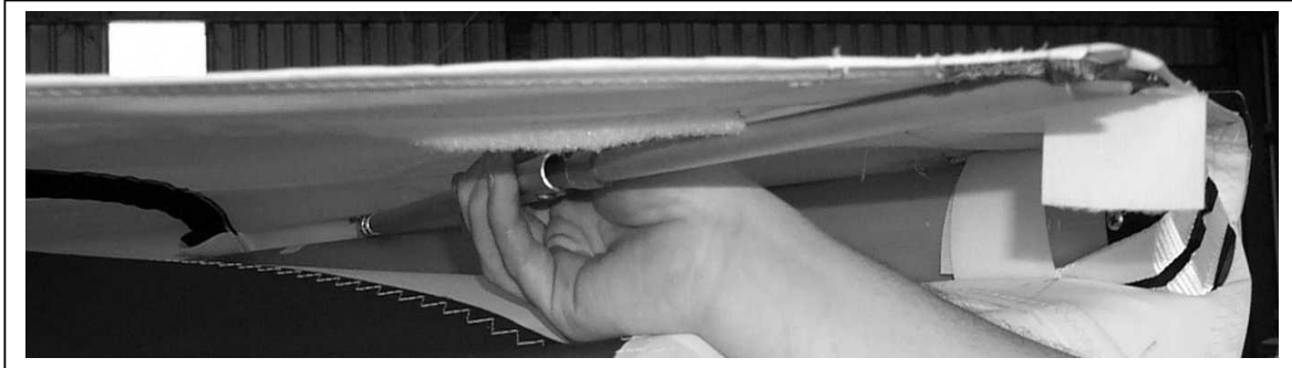
Figure 13 Section 4. Load Tip Strut
