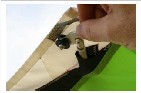
Figure 59 Section 4. Unload Over-Centre Tip Battens
