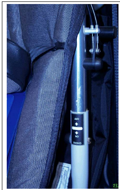
Figure 6 Section 2. Choke Placard Location (Under Seat Bag Placard in Background)
