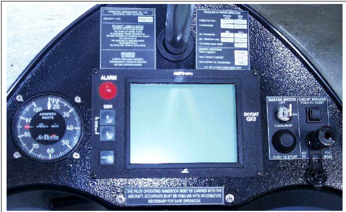
Figure 1 Section 2. Flight Limitations, Airspeed, Circuit Breaker, Power Socket and Operators Handbook Placard Locations
