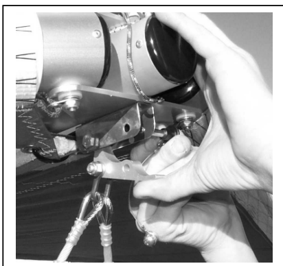
Figure 49 Section 4. Disconnect Nose Catch and Remove Nose Cone
