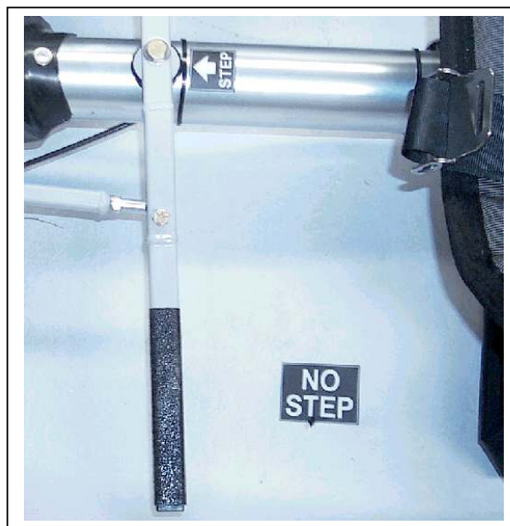
Figure 7 Section 2. Step and No Step Placards
