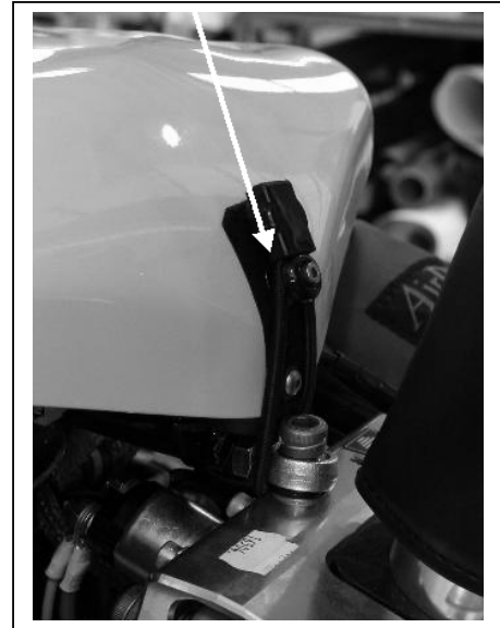
Figure 39 Section 4. Engine Cowl Retention Rubber Cord
