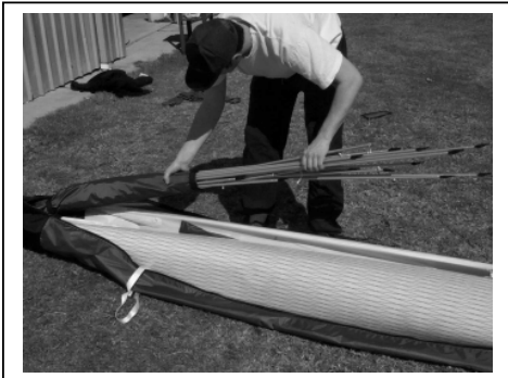
Figure 74 Section 4. Position Battens
