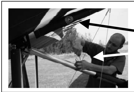
Figure 31 Section 4. Attach Trimmer to Mast
