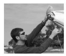
INSERT NOSE BATTENS. Insert the nose battens tail end first and locate them on the fittings on the front of the keel.
