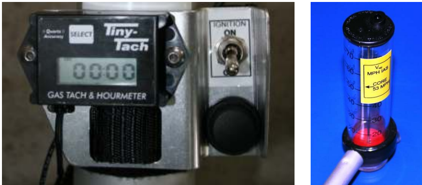
Figure 2 Section 9. Digital Instrument Panel (Tiny Tach & Hall airspeed indicator)
