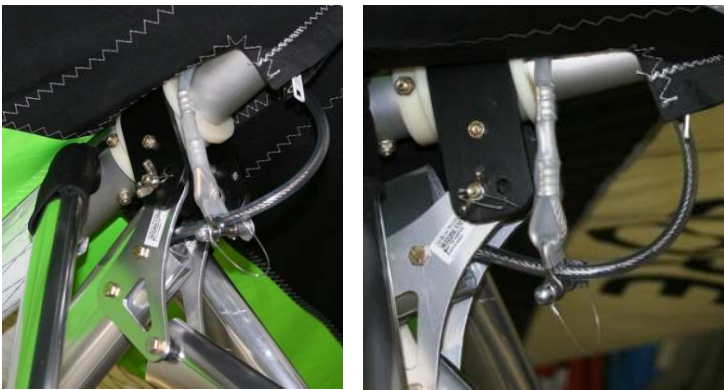
Figure 15 Section 4. Attaching the back up loop
