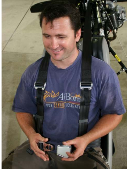
Figure 2 Section 7. Restraint harness, shoulder sash & buckle fitting.
