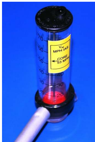
Figure 6 Section 7. T-Lite airspeed indicator.
