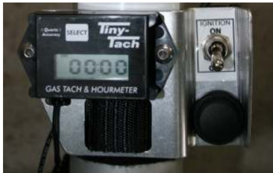
Figure 5 Section 7. T-Lite rpm / hour meter.
