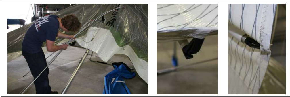
Figure 6 Section 4. Insert main sail battens
