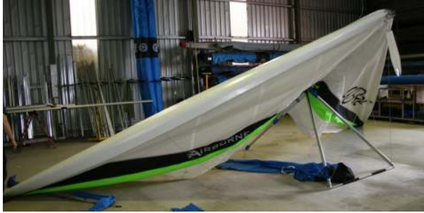
Figure 4 Section 4. Spreading the leading edges
