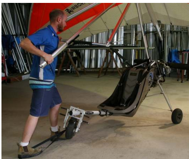
Figure 18 Section 4. Lifting and rotating the wing onto the base
