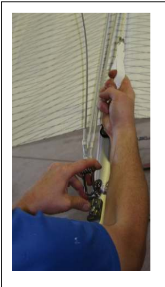
Figure 27 Section 4. De-tension pullback cable
