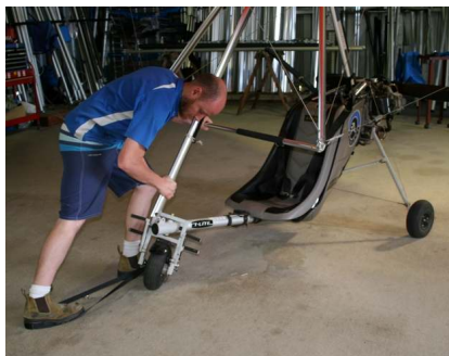
Figure 18 Section 4. Lifting and rotating the wing onto the base
