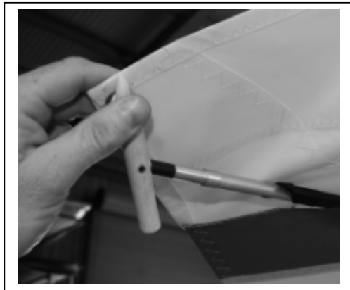
Figure 23 Section 4. De-tension tip strut
