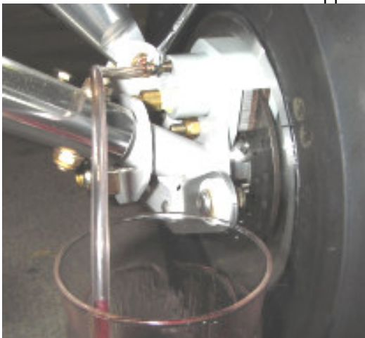
Figure 45 Bleed Drain Hose Connected
