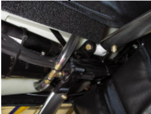
Figure 46 Inspect All Junctions for Oil Leakage
