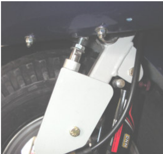
Figure 38 Rear Disk Brake Master Cylinder Mounted on Front Fork
