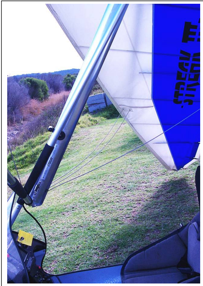
Figure 13 Securing of Base Bar with Shock Cord
