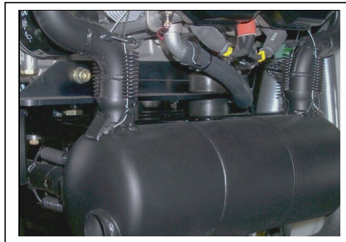
Figure 26 Muffler Safety Wire and Springs
