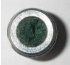
Figure 39 Cap Grit Plug, Remove the Plug from the Grub Screw for Allen Key Access.
