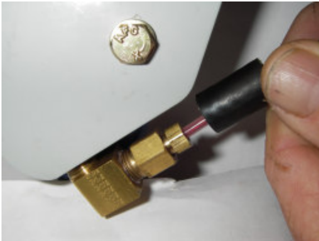
Figure 43 Master Cylinder, Push Triple Sleeving Over the Compression Fitting Nut
