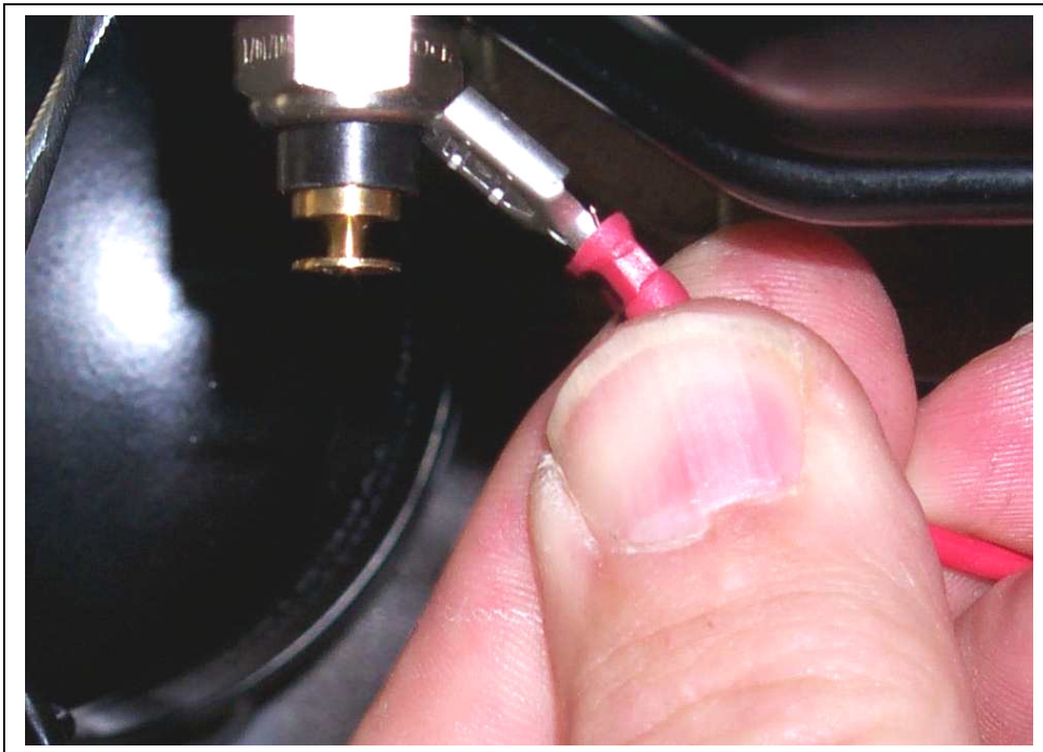
Figure 77 Earthing of CHT Sender, to Check the Wire to the SkyDAT.
