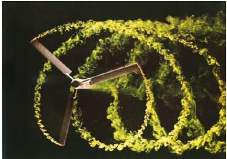
The rotor tip vortices, shown above with a 3-blade rotor example, continually peel or strip away from each blade in a process known as tip-vortex shedding. In humid conditions these small diameter tip vortices are sometimes visible in helicopters as thin wispy foggy ribbons moving downward.
