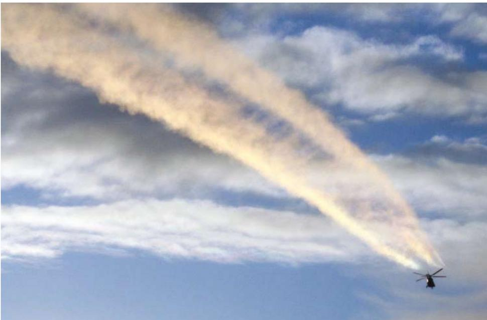
These parasitic swirling disk vortices involve significant portions of the wake or downwash spiralling wastefully upward again in a swirling horizontal funnel on each side of the core wake. The vortices contribute significantly to the overall drag of the machine. Another way of considering disk vortices is that they steal energy created by the engine and convert it uselessly into two horizontal funnels of energized air.
